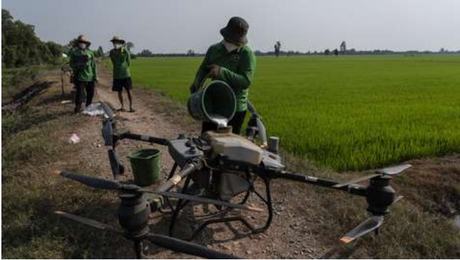
A worker loads fertilizer into a tank attached to a large drone, preparing to spray it rice fields in Long An province in southern Vietnam's Mekong Delta, on January 2
